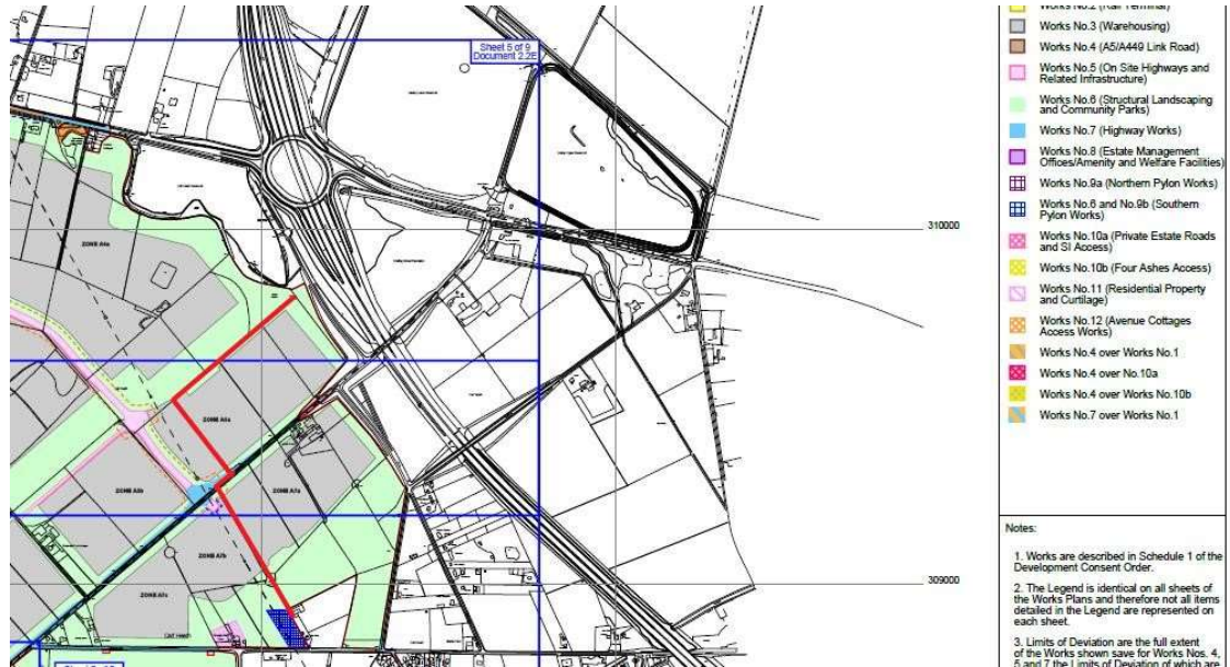
Fig 4.3: Doc 2.2 TR050005-000219 - Works Plan showing Inglewood Investment Land Boundary and Highways and Infrastructure works
